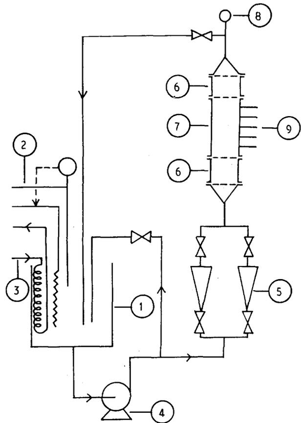
Figure 2 Experimental equipment (1, storage tank; 2, contact thermometer coupled with a regulated heating resistance; 3, water refrigerator; 4, centrifugal pump; 5, flowmeters; 6, calming sections; 7, bed packed with foam; 8, temperature probe; 9, pressure taps).
