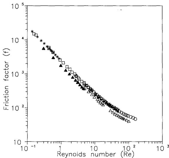
Figure 3 Experimental data concerning flow-through configuration. Foam g 45: (○) water, (□) glycerol. Foam g 100: (☆) water, (\*) glycerol, (★) air. Foam g 60: (Δ) water, and (▲) glycerol.
