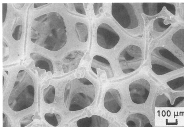
Figure 1 Scanning electron micrographs of nickel foam (Grade 60).
